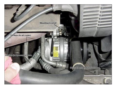
The low pressure hose needs to be removed and remade to correct length using the provided fitting with new thread size. Utilize your local a/c shop for this: about \$10.00. The high pressure hose can utilize the existing fitting.
