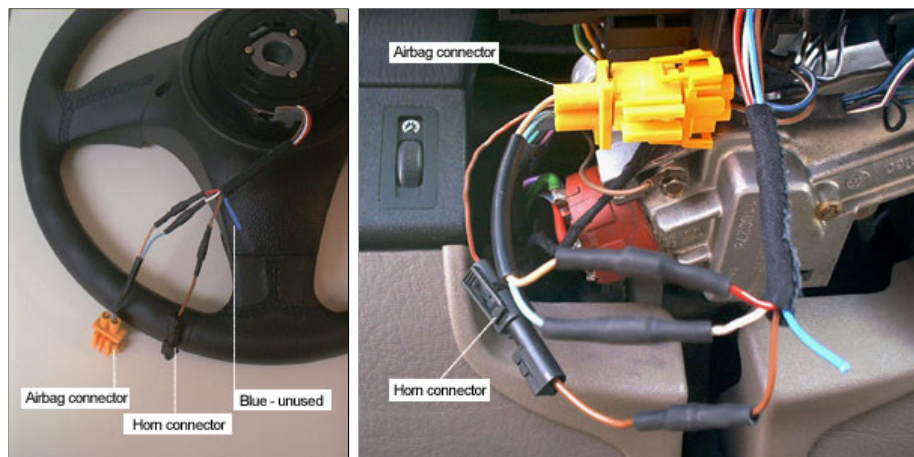
Connections and heat-shrink tubing in place. Note wire color combinations
